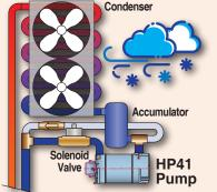
When the outside temperatures become low enough to maintain the desired cooling temperature, there is no need to compress the refrigerant to a higher pressure/temperature.
