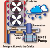
When the outside temperatures become low enough to maintain the desired cooling temperature, there is no need to compress the refrigerant to a higher pressure/temperature.
